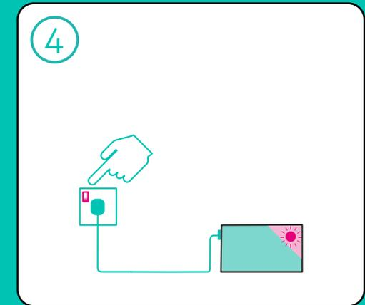
Connect the adapter to the base unit, plug into a wall socket and turn the power on at the wall. The base will beep and lights flash twice.
