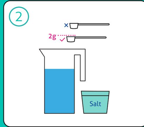
Add 2g of table salt - that's a flat measure using the measuring spoon provided. No more or less as this affects the electrolysis. If too much salt is added, rinse out the jug and start again. Do not use rock salt.
