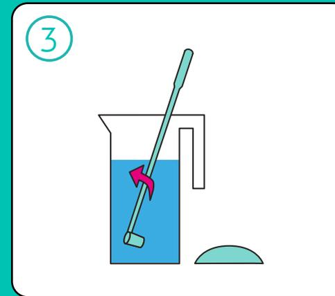
Stir the solution at least 8 times in the centre of the jug to fully dissolve the salt. The salt acts as an electrolyte and if it accumulates on the electrode the product will not work. Place the lid on the jug, and wipe any water away from the electrodes on the bottom of the jug.
