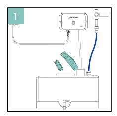
Unscrew the tank's black lid and add one soluble salt sachet. There shouldn't be any water in the tank at this stage.
