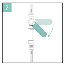
Open the lever valve to fill the tank up to the 10 litre mark. If the unit isn't plumbed in simply fill by hand.
