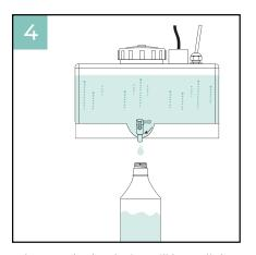
When ready, the device will beep, light turns green and you have 10 litres at 100ppm in the tank. Use the tap to dispense the solution into bottles or buckets.
