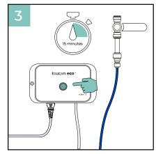
Switch on the activator unit - the unit's light will turn green. Press the button, the light turns blue and the electrochemical activation begins. This will take 15 minutes, during which time you will see bubbles around the cell and a faint smell of chlorine once activated.
